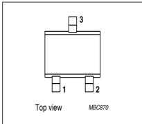
Fig.1 Simplified outline (SOT323) and pin configuration.
