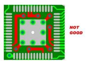
Routing and vias between the flag and the pads can easily be shorted to either the flag or to the pads because of the physical dynamics of the solder under the device. Shorts can occur to traces and, especially, to vias even if they are covered by soldermask. This is because the trace edges (crowns),
