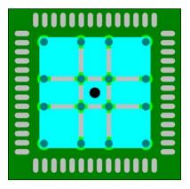
Consider the size, quantity, position, and type (tented, plugged, open, etc.) of vias used within the flag to determine their effect on the amount of solderpaste the may be wicked from the pad by the vias during soldering and make appropriate adjustments to the stencil openings and via positions.
