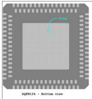
QFN packages generally have a row (QFN) or two (DQFN) of perimeter pads ("pads") around a larger central pad ("flag" or "Epad") encapsulated in a plastic body. These packages are surface-mounted to the target system PCB by a solder reflow process. All of the SMSC QFN and DQFN packages are like this.
