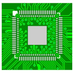
It is usually desirable to breakout the inner pads of a DQFN to the inside and drop vias to escape the part. Per the discussion above, this can cause shorts under the device, but the  $\underline{D}$ QFN devices have a larger gap between the pads and the flag, making this problem less likely.
