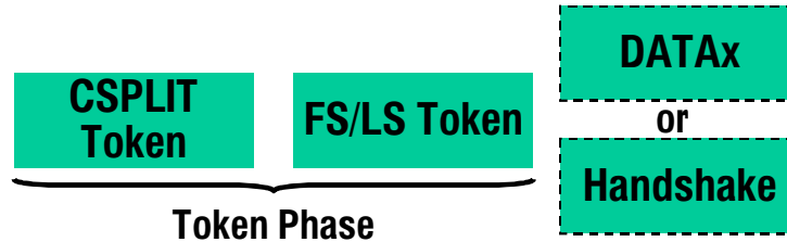
Figure 8-7. Packets in a Complete-split Transaction
