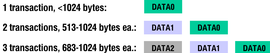
Figure 5-11. Data Phase PID Sequence for Isochronous IN High Bandwidth Endpoints
